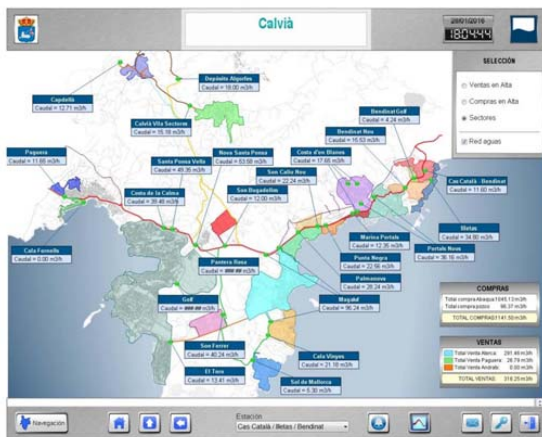
Pantalla general TELECONTROL
